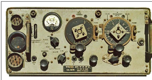
Wireless Set No. 19 (here shown the British Mk.II model, set without power supply unit). Use: primarily developed for AFVs but later used as a general purpose set. Frequency range 'A' set 2-8MHz; 'B' set 229-241MHz. MO control. R/T, MCW, CW. RF output 'A' set 1.2-2.5W (R/T). Range 'A' set up to 15 miles; 'B' set \frac{3}{4} mile.
