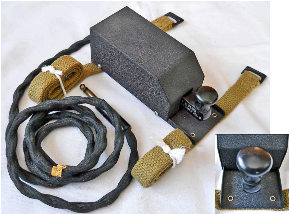
Key and Plug Assembly No. 9 ver. 9.1 was produced in the U.S.A. by J.H. Bunnell. Most significant differences to the British parent assembly were a type PL-55 plug and a smaller key knob.
