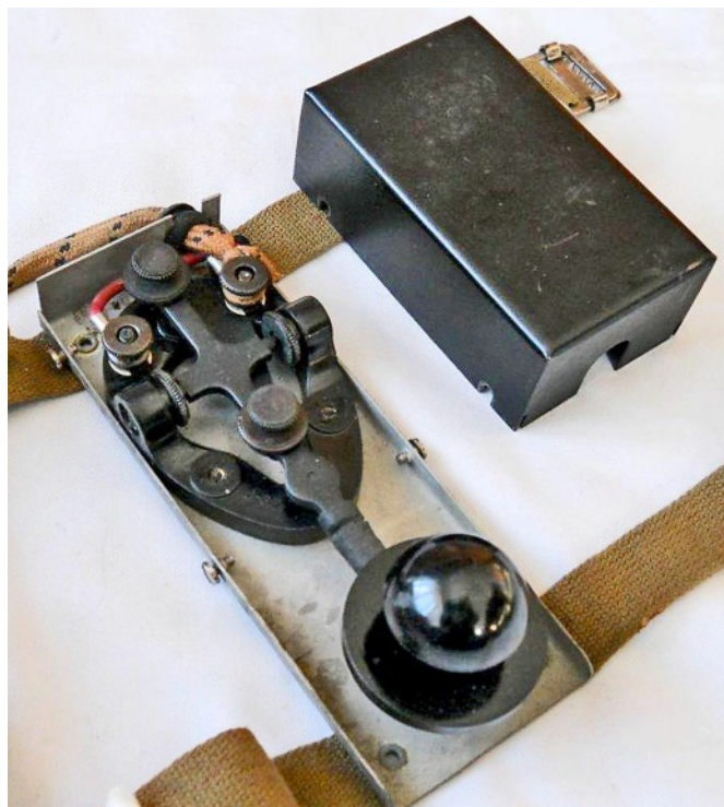
Internal view of Key and plug Assembly No. 9 ver. 10.2 showing a modified type J-37 key with black finish hardware. For more details see page 35.
