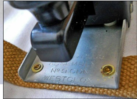
Front view of the No. 9 Type 2 assembly showing a slightly different key lever insulation sleeve (below).
