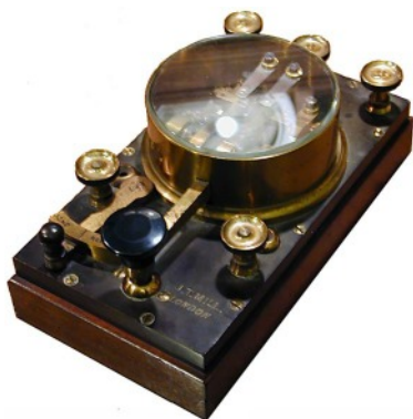
British General Post Office double current Morse key (one of the many versions).
