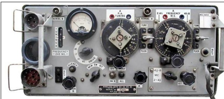
Wireless Set No. 19 Mk.II produced by RCA in the USA. Use: primarily developed for AFVs but later used as a general purpose set. Frequency range 'A' set 2-8MHz; 'B' set 229-241MHz. MO control. R/T, MCW, CW. RF output 'A' set 1.2-2.5W (R/T). Range 'A' set up to 15 miles; 'B' set \frac{3}{4} mile.
