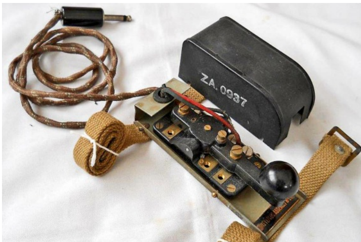
Internal view of Key and Plug Assembly No. 9 ver. 3.3 with Key W.T. 8 Amp No. 2 Mk.III (left) and front view showing the lacquered identification plate (right).
