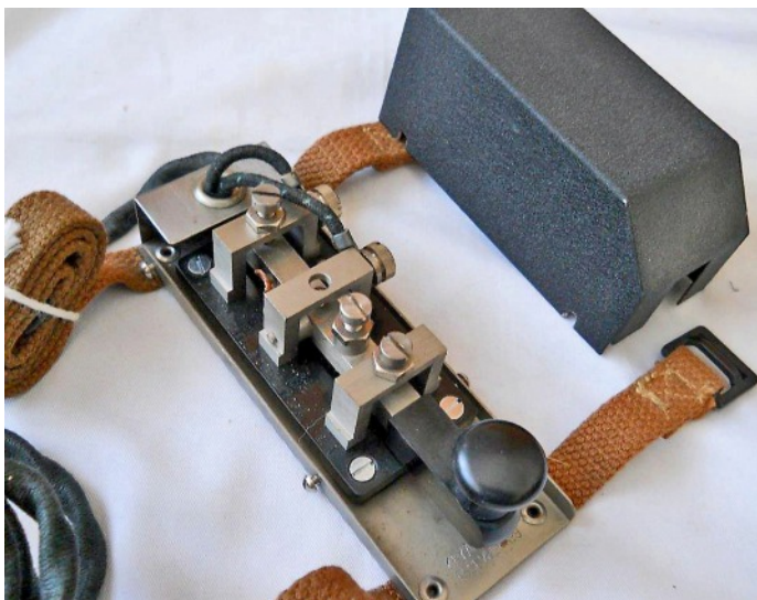
Key and Plug Assembly No. 9 ver. 9.2 had a plated assembly base plate and a black wrinkle finished protective cover. The Key W.T. 8 Amp No. 2 had three bridges.
