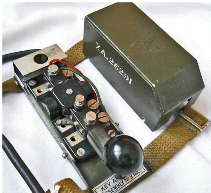
Front view of Key and Plug Assembly No. 9 Mk.I/I (above) and with protective cover removed (right). Note that all the brass parts of the Key W.T. 8 Amp No. 2 Mk.III and the plug were plated.
