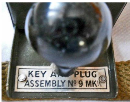
Front view of Key and Plug Assembly No. 9 Mk.I/I (above) and with protective cover removed (right). Note that all the brass parts of the Key W.T. 8 Amp No. 2 Mk.III and the plug were plated.
